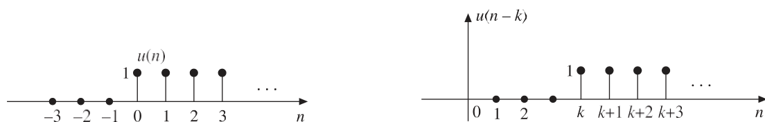
Figure 1.3 Discrete-time (a) Unit step function (b) Shifted unit step function
